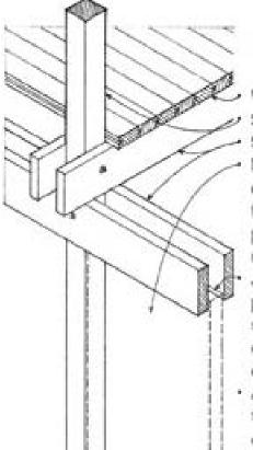
Wood decking; see 4.40. Solid column Spaced beams
