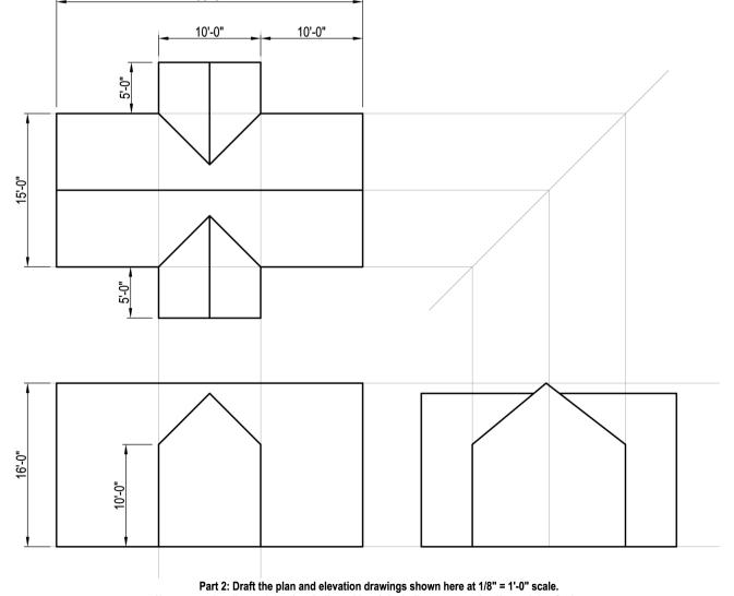
Use appropriate line weights (not indicated here), including construction line weights for layout. Note: More construction lines are required than are displayed here.
