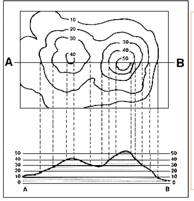
Contour lines are drawn on a map to connect points of equal elevation.
